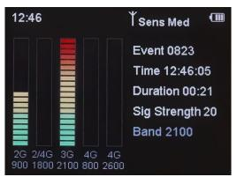
Live Cellular Mode showing two detected signals
